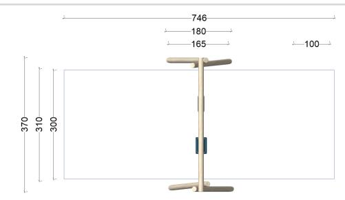
Robinia pillars are curved - widen the swings' legs if necessary for the installation of the upper beam.
